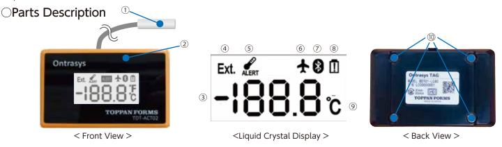
①External temperature sensor (BDT01-LC40:Semiconductor sensor / BDT01LC196:Platinum sensor) ②LED ③Temperature display ④External temperature ⑤Alert ⑥Airplane mode ⑦Usual mode ⑧Low battery alert ⑨℃ ⑩Mounting screws
